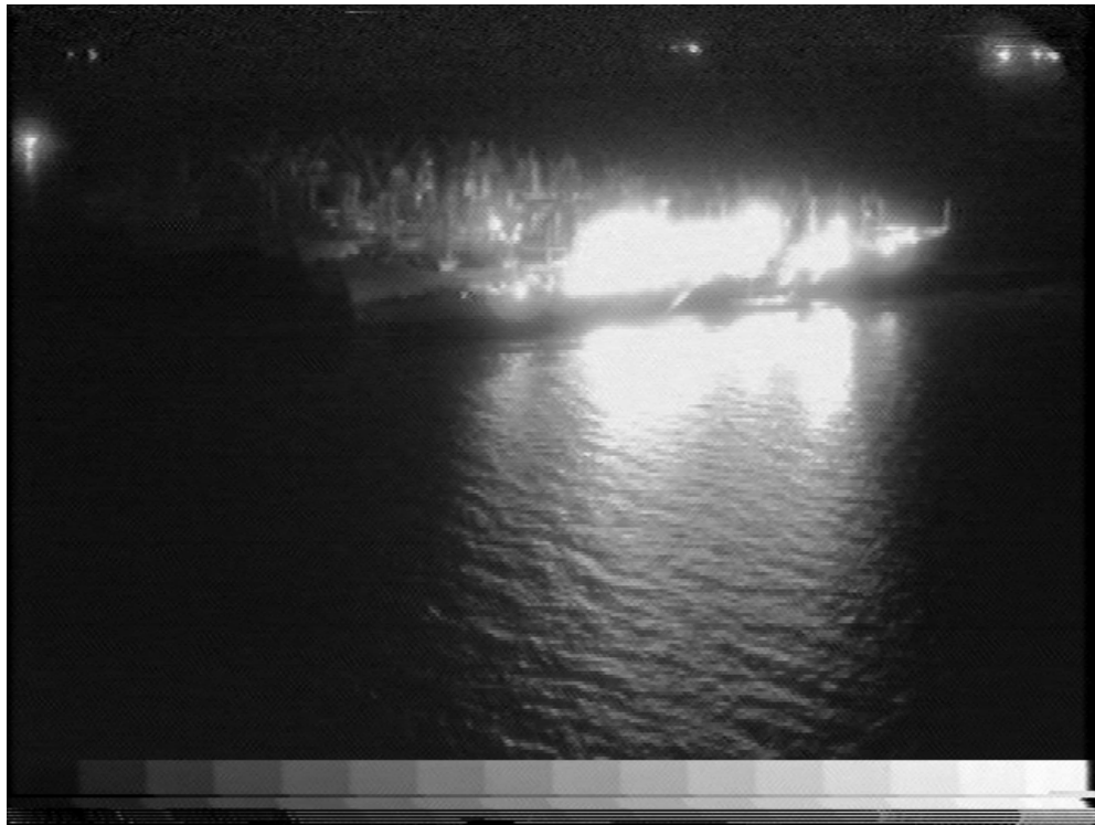
Figure 8: An II image degraded by over-exposure [From NRL].
