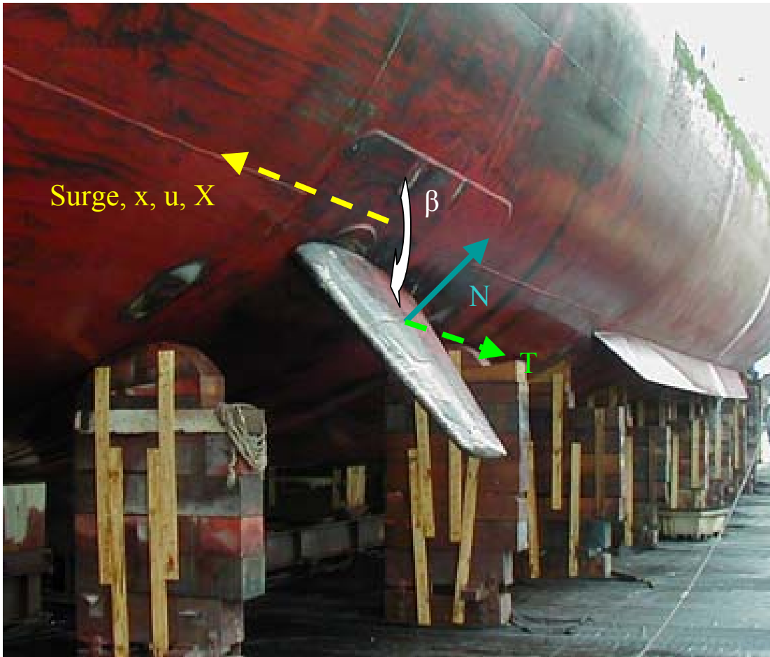
Figure 6. Fin Stabilizer Forces and Moments.
