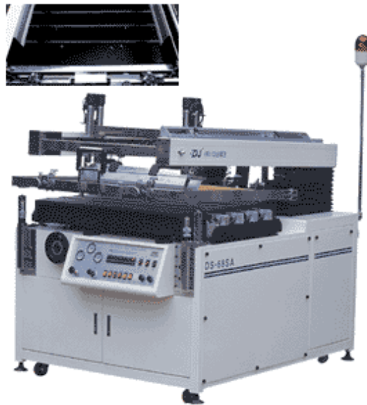
Figure 50: Typical screen printing machine for printing on flat surfaces.
