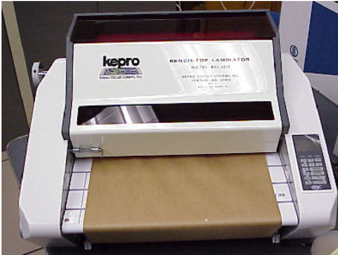
Figure 33: Kepro desktop roll type laminator.
