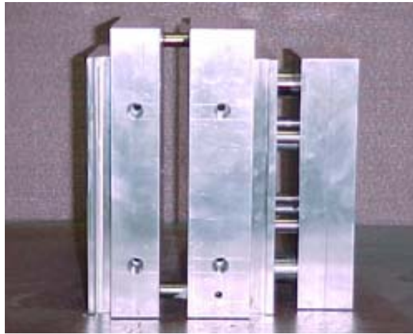
Figure 38: The molds plates used for Injection molding.
