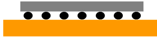
Flip chip without underfill material
