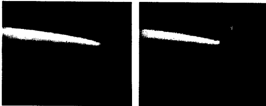
(a) Before breakdown (b) After breakdown Fig. 1 In-situ observation of both electrodes before and after the electrical breakdown.
