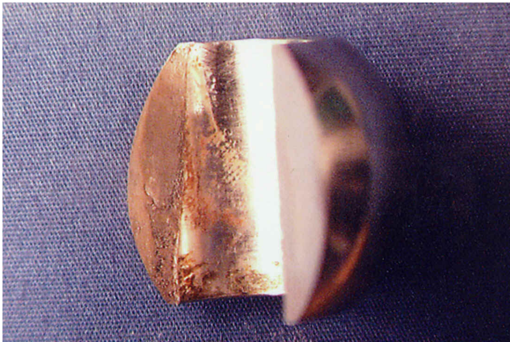
Figure 7. Fracture half “B” depicting corrosion along the inside bore (mag ~2x).
