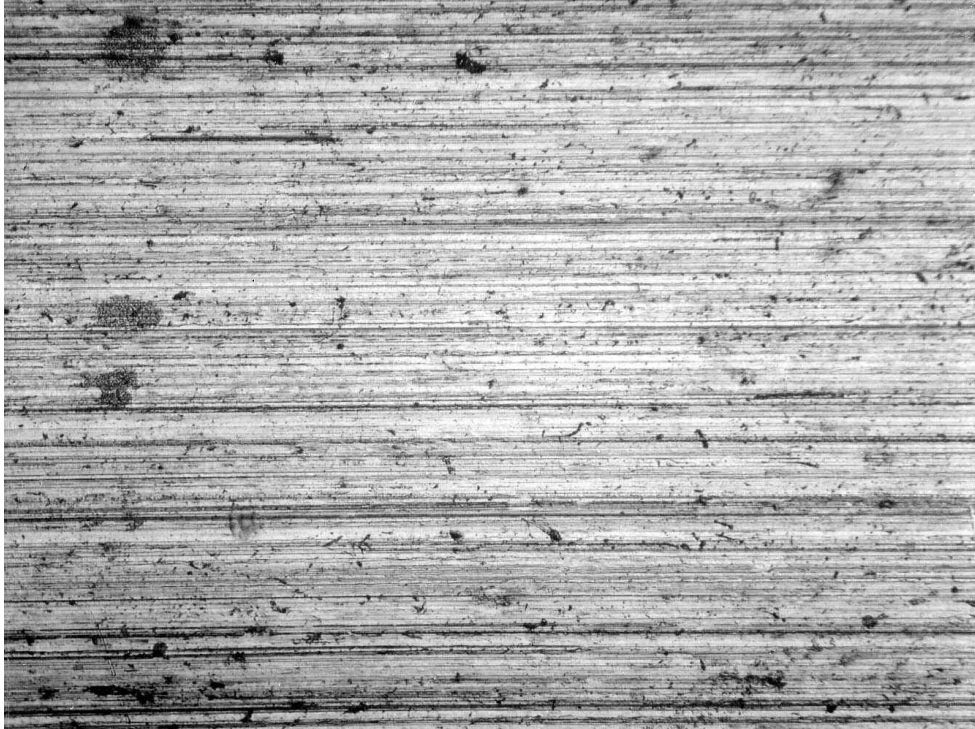
Figure 57. Macrograph of machined surface of rod end fitting ball (mag. 100x).
