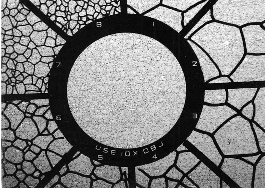
Figure 24. Etched microstructure demonstrating the grain size to be 8 or finer (mag 100x).
