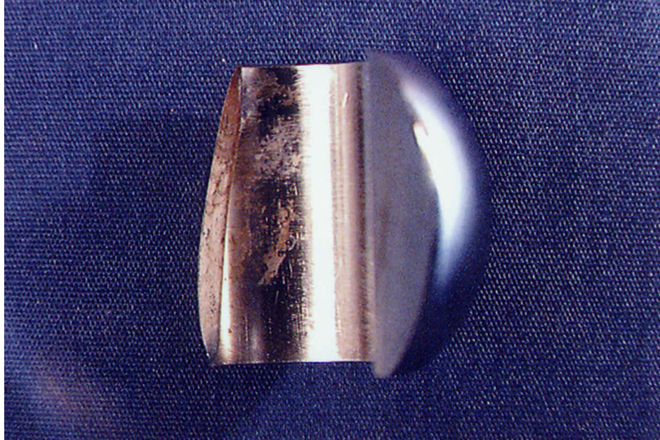
Figure 6. Fracture half “A” showing corrosion along the inside bore (mag ~2x).
