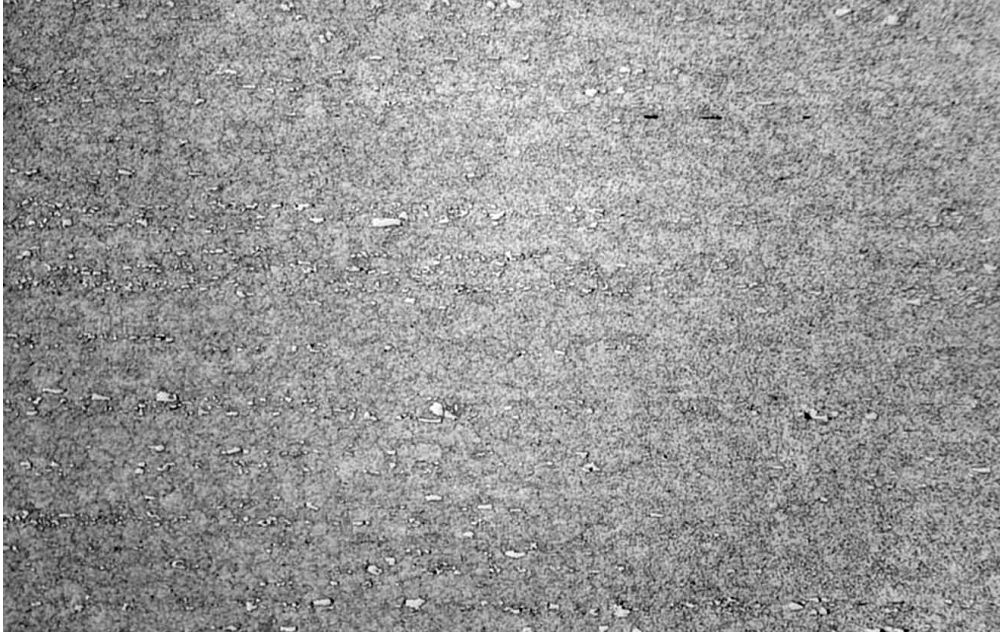
Figure 23. Etched microstructure of the ball material showing the presence of banding (mag 100x).
