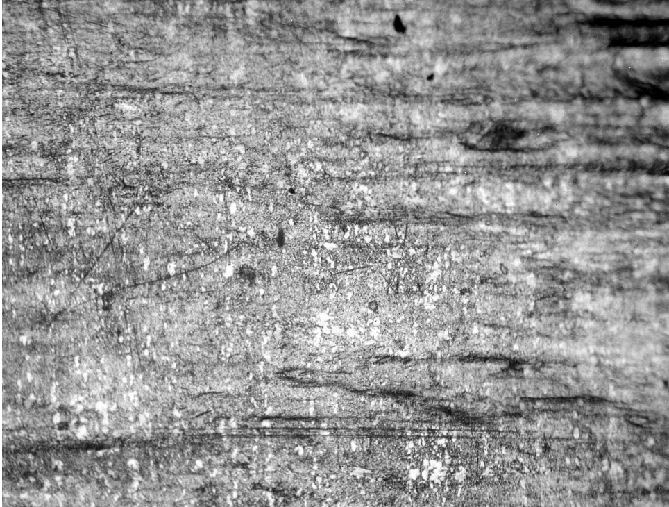
Figure 56. Macrograph of as-received surface of rod end fitting ball subjected to sensitization testing (no inter-granular attack was noted) (mag. 100x).
