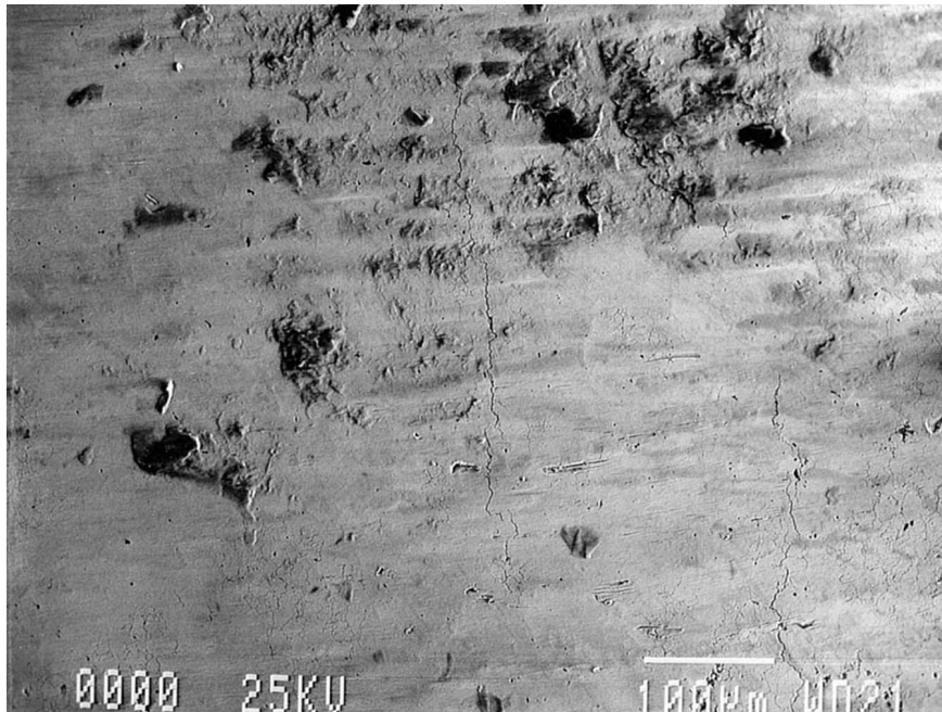
Figure 46. Secondary cracks near and parallel to the fracture surface (mag. 150x).
