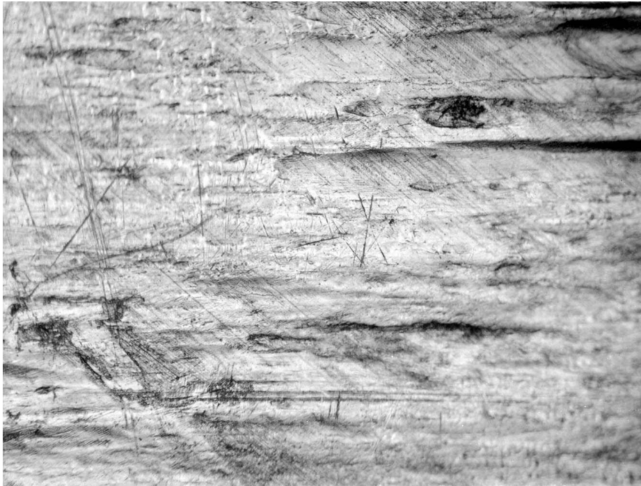
Figure 55. Macrograph of as-received surface of rod end fitting ball (mag. 100x).
