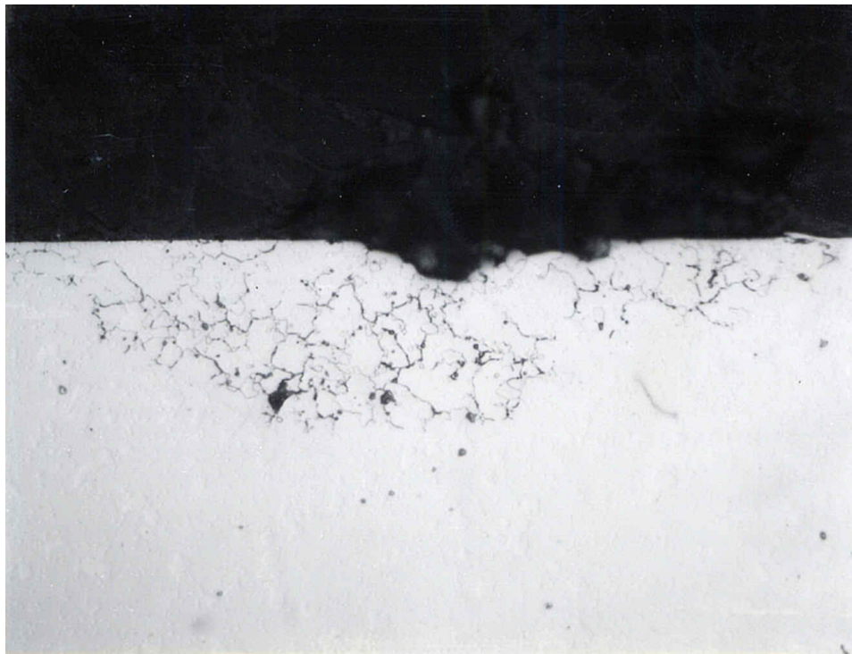
Figure 18. Transverse metallographic section area "B," unetched (mag 500x).
