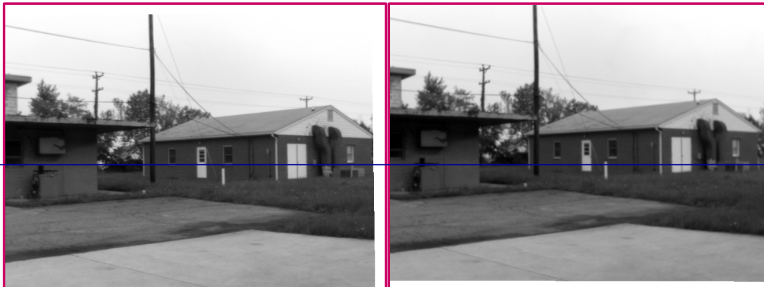
Figure 28. Rectified image pair for the building image pair with calibration image set 2 parameters.
