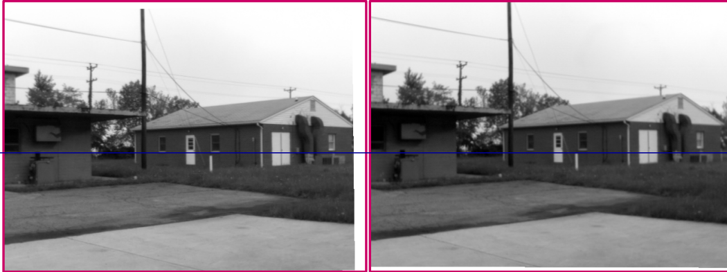
Figure 30. Rectified image pair for the building image pair with calibration image set 4 parameters.
