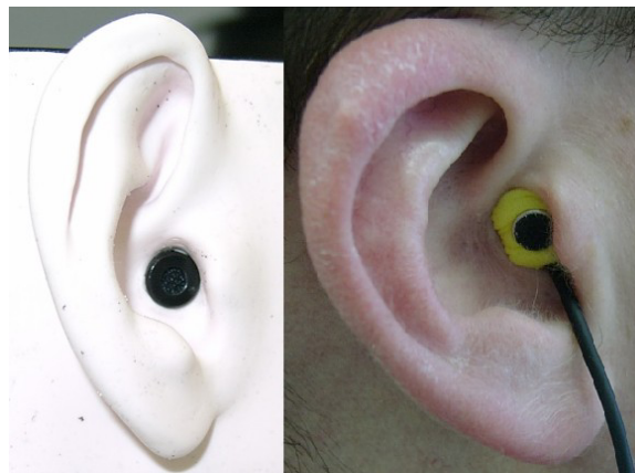
Figure A-9. The local user places the microphone facing out, using the pre-fabricated earplugs designed for holding the microphone.
