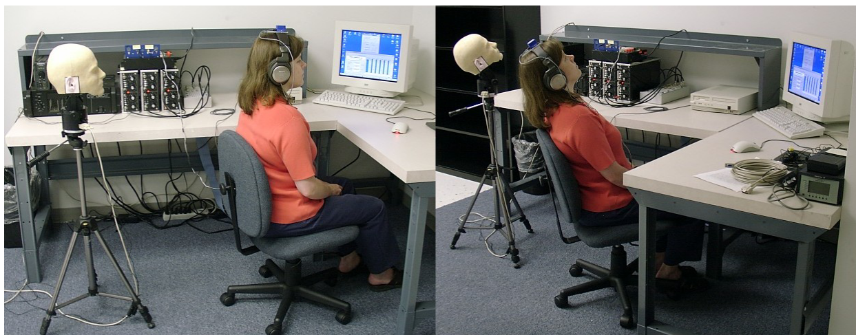
Figure 17. Fully functional wired binaural microphone system.
