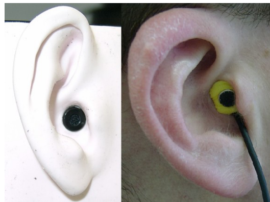
Figure 6. Sensing microphone in the artificial ear (left) and identification micro-phone in the human ear (right).
