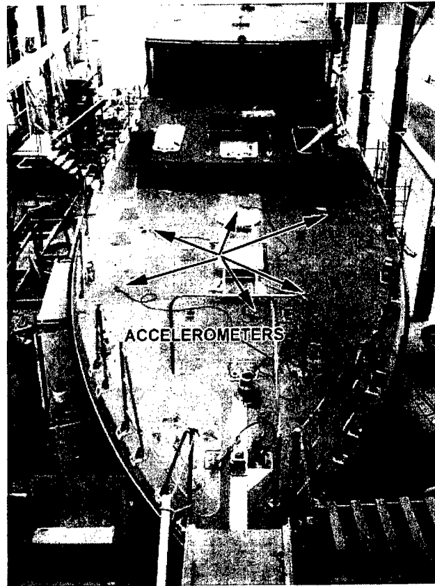
Figure 5. Accelerometer Positions Are at the Head of Each Arrow
