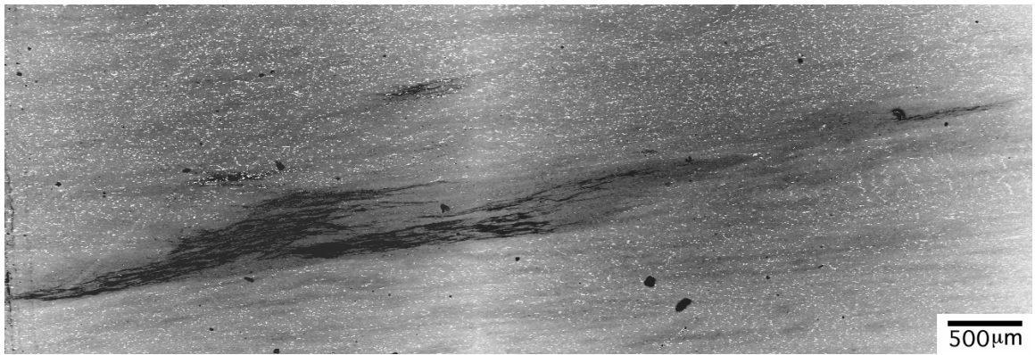
Figure 5, Back scattered SEM image of a low density segregation defect in KD-CBS .
