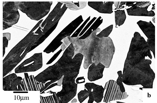
Figure 6: Regions containing globular-type high-density phases, a) Low magnification highlighting large amount of beta phase (BEI), and b) high magnification showing small volume fraction of lamellar phase within globular region (BEI).
