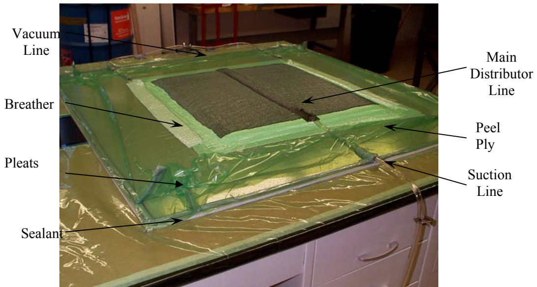
Figure 24. Approach With the Main Distributor in the Middle of the Panel
