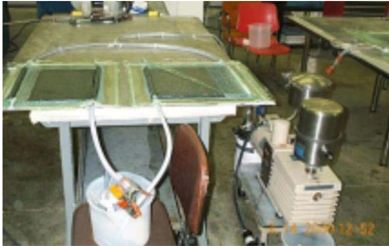
Figure 1. Fabrication of Laminate by VARIM Process
