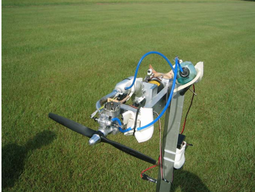
Figure 23. Engine Mounted on Test Stand 4 Feet Above Ground
