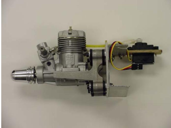
Figure 19. Engine Mounted on Dubro Vibration Reducing Motor Mount
