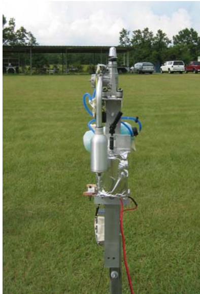
Figure 16. Engine Mounted on Test Stand 5 Feet Above Ground
