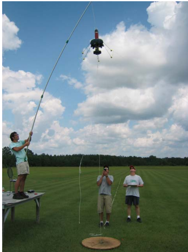
Figure 18. VTOL UAV Tethered 15 Feet Above the Ground
