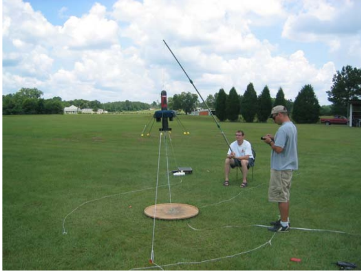
Figure 15. VTOL UAV Tethered 5 Feet Above the Ground
