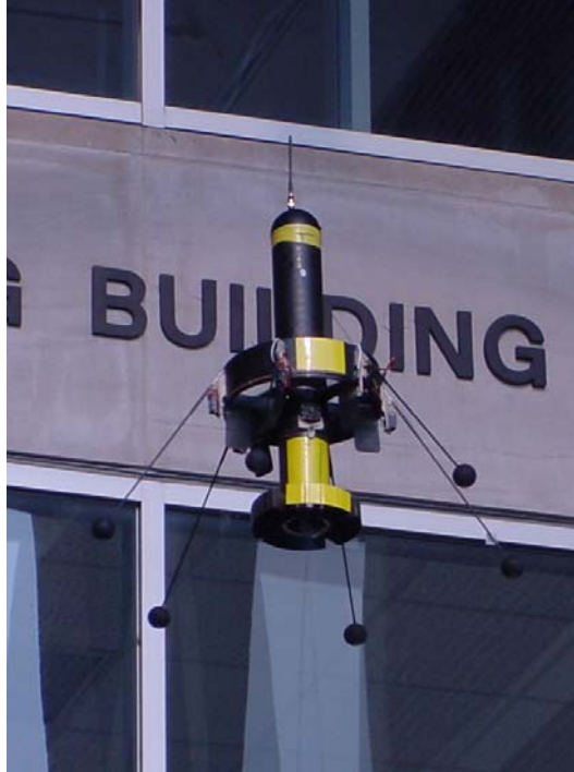
Figure 1. Auburn University/ Micro Autonomous Systems VTOL Ducted Propeller UAV
