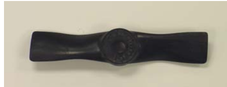
Figure 7. Modified Master Airscrew 11 X 5 Cut Down to a 4 11/16 X 5
