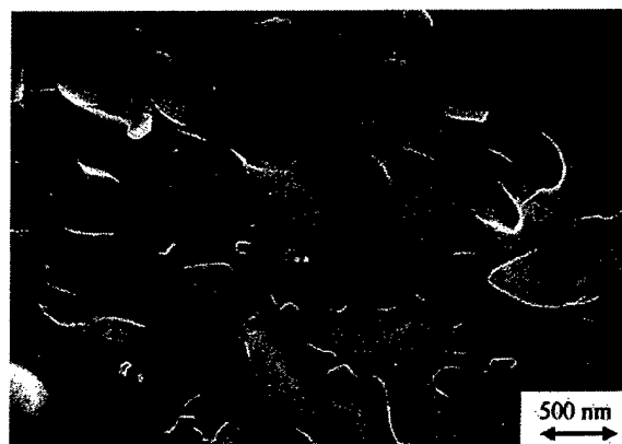
Fig. 10. SEM micrograph of the fracture surface of a fiber crept at 1400^\circ \text{C} . It can be seen how cracks propagate preferentially at the interfaces (arrowed). Damage is also probably nucleated at the interfaces due to the high shear stress associated to the different elastic and plastic properties of alumina and garnet phase.
