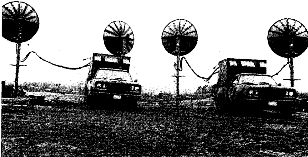
A TRC-97A troposcatter radio relay element is set up to provide TACS unit tactical communications connectivity. (USAF photo.)
