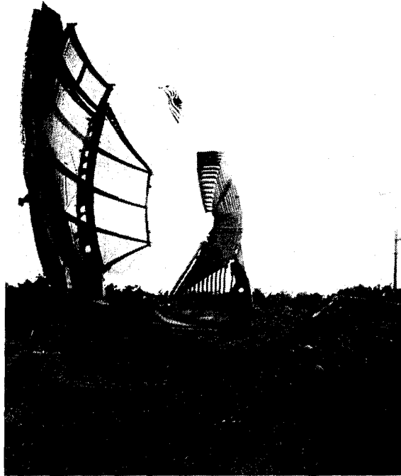
AN/TPS-43 radar, the mobile sensor of the tactical air control system, after setup and camouflage during a tactical air control system deployment. (USAF photo.)
