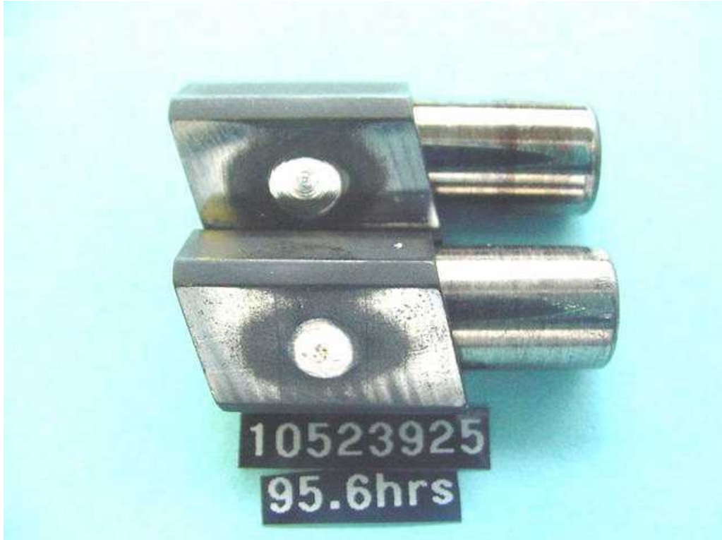
Figure 12. Test 1 Pump 1: Shoe Back and Roller Wear
