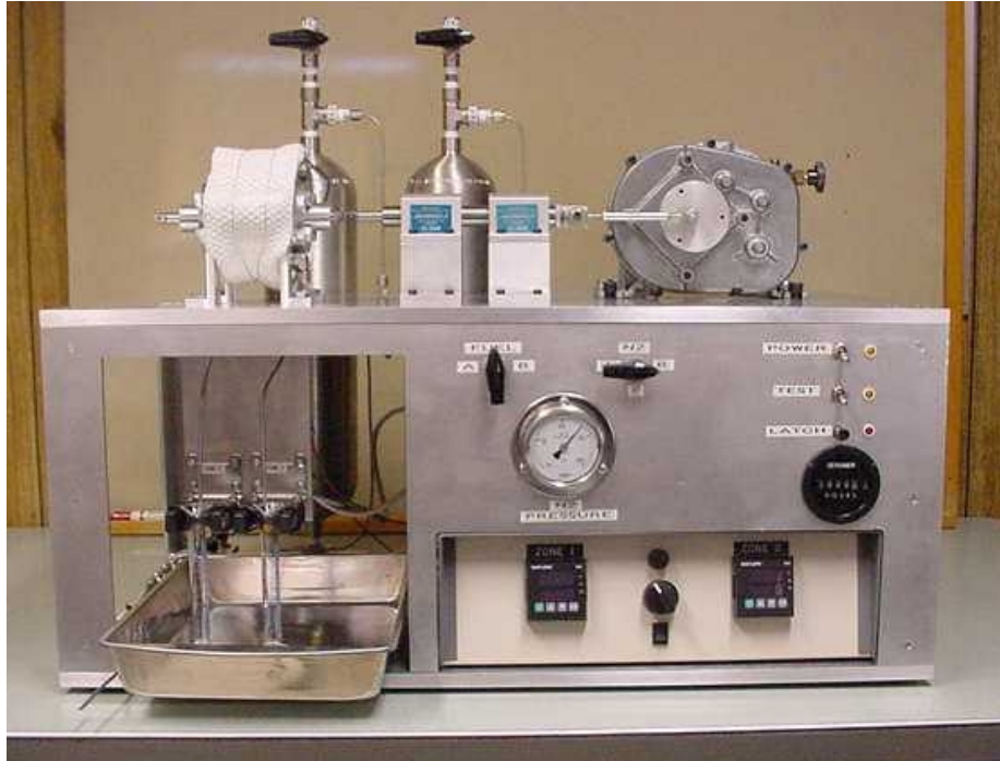
Figure 2. Face on view of Dynamic Seal Test Rig. Axial motion of the shaft within the heated block is supplied by a bell crank mechanism and cross-head assembly.
