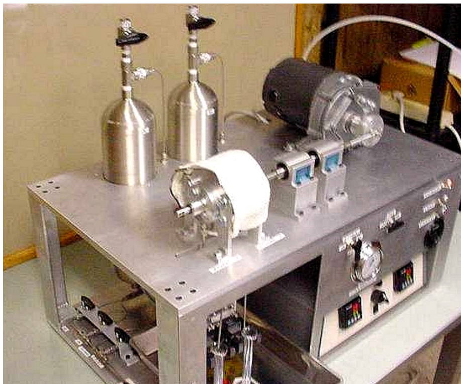
Figure 3. View of top surface layout of Dynamic Seal Test Rig. Two fuel reservoirs are available for testing with two different fuels.
