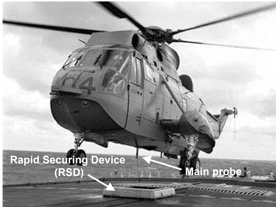
Figure 2: Helicopter hovering over RSD, hauldown wire attached.
