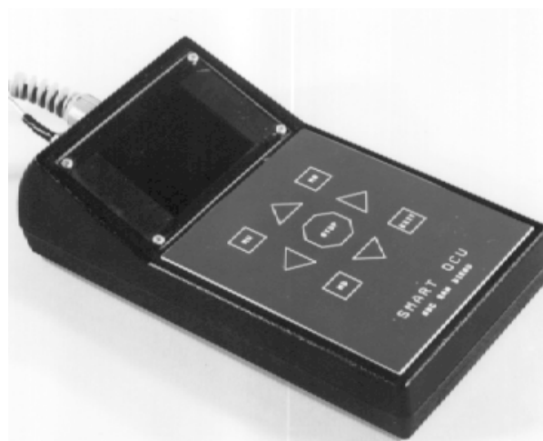
Figure 4. The initial MPRS control pendent employed an integrated 2.5-inch video display and capacitive touch pad for semi-hands-free operation.
