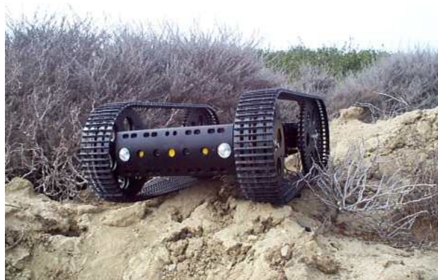
Figure 2. Front-mounted Sensor Snout showing the dual headlights, Sharp I/R arrays, and three forward sonars.
