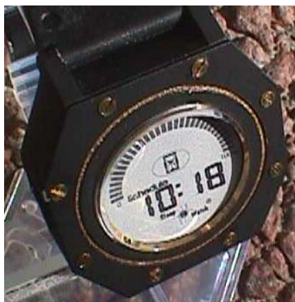
Figure 7: Sleep Watch Actigraph showing Fuel Gauge-Type Current Performance Capacity Readout.
