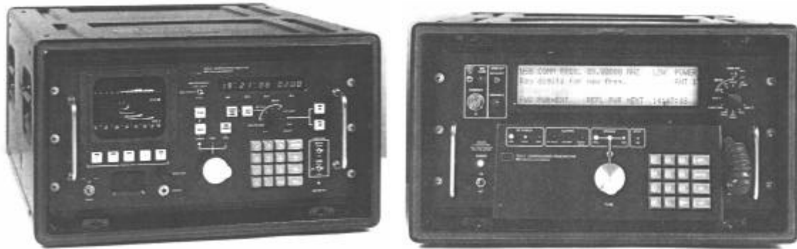
Figure IV-13. AN/TRQ-42 Transmitter and Receiver
