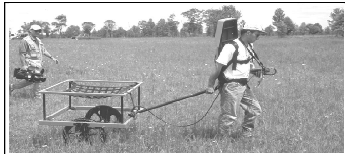
Figure 13. Typical EM Induction System
