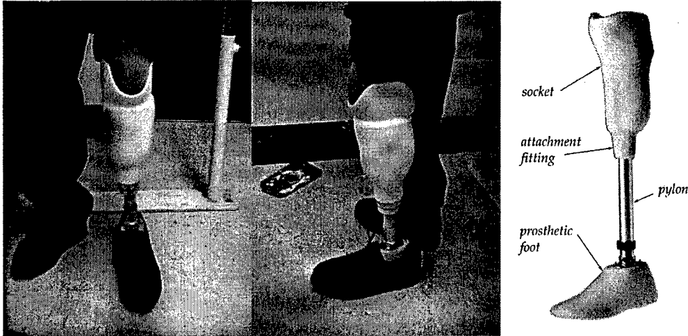
Figure 1: On the left and center, a patient testing an SLS fabricated socket; on the right, the description of the parts of a prosthesis for below-the-knee amputees.
