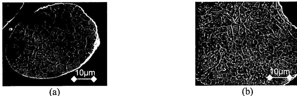
Figure 8. Microstructure of gas atomised H13 <150/+75µm size fraction
