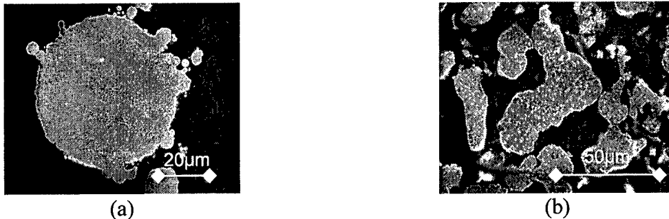
Figure 3 Microstructures of M2 powders. (a) Gas atomised <150/+75 . Note the fine carbide network. (b) Water atomised <38\mu\text{m} fraction. Note fine discrete carbides.
