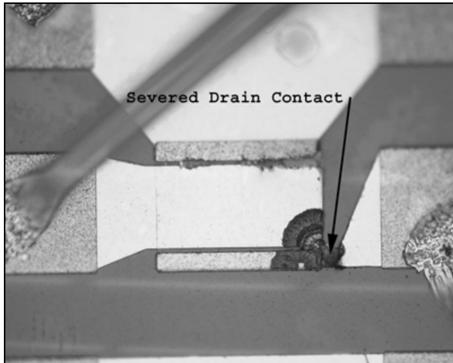
Figure 63. Sample A0315 FatFET Irradiation Experiment Drain Damage
