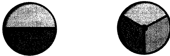
Figure 12. Partitioning of an element into two (left) or three (right) segments to allow electronic steering of the beams.
