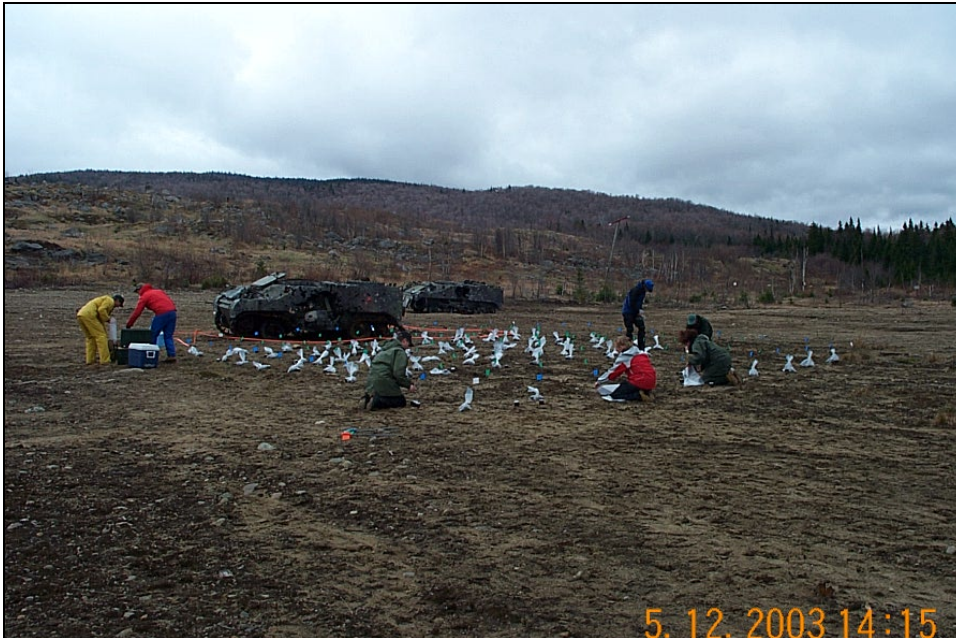
Figure 21. Collecting discrete and composite soil samples in Grid 10.
