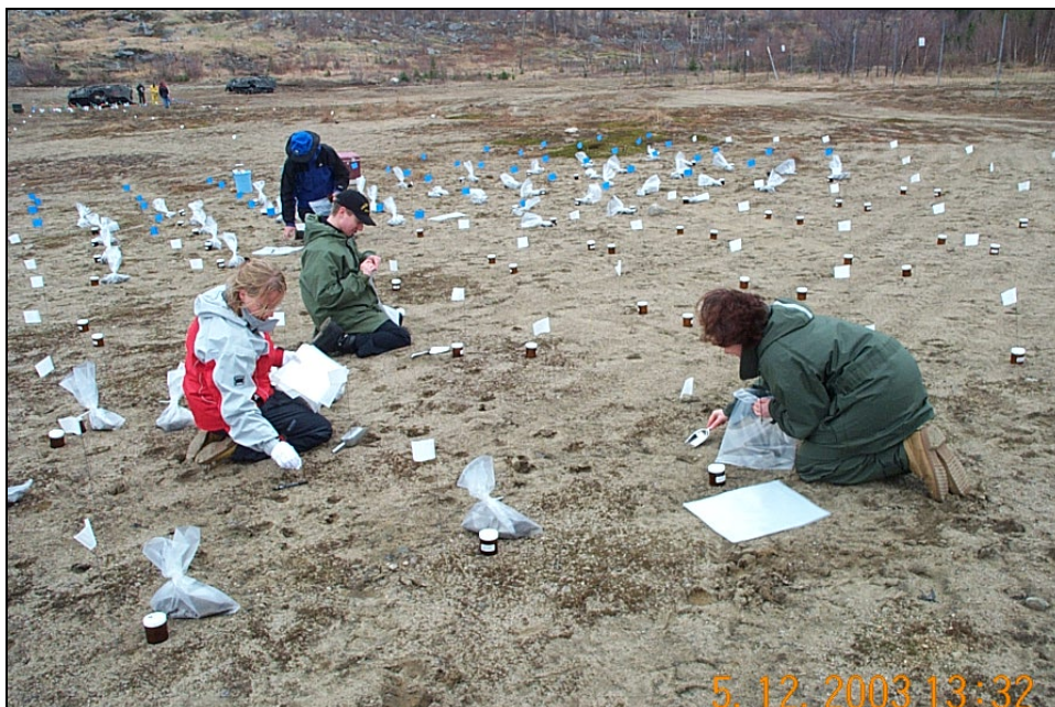
Figure 8. Discrete and composite soil sampling in Grid 3.
