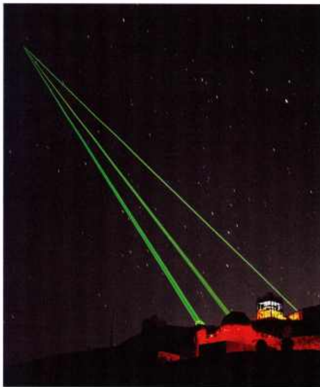
Kirkland AFB, NM—The Air Force's Starfire Optical Range uses three laser beams to accurately measure rapid changes in the earth's atmosphere. This data is used to maximize the power and range of the developmental Airborne Laser Program.
