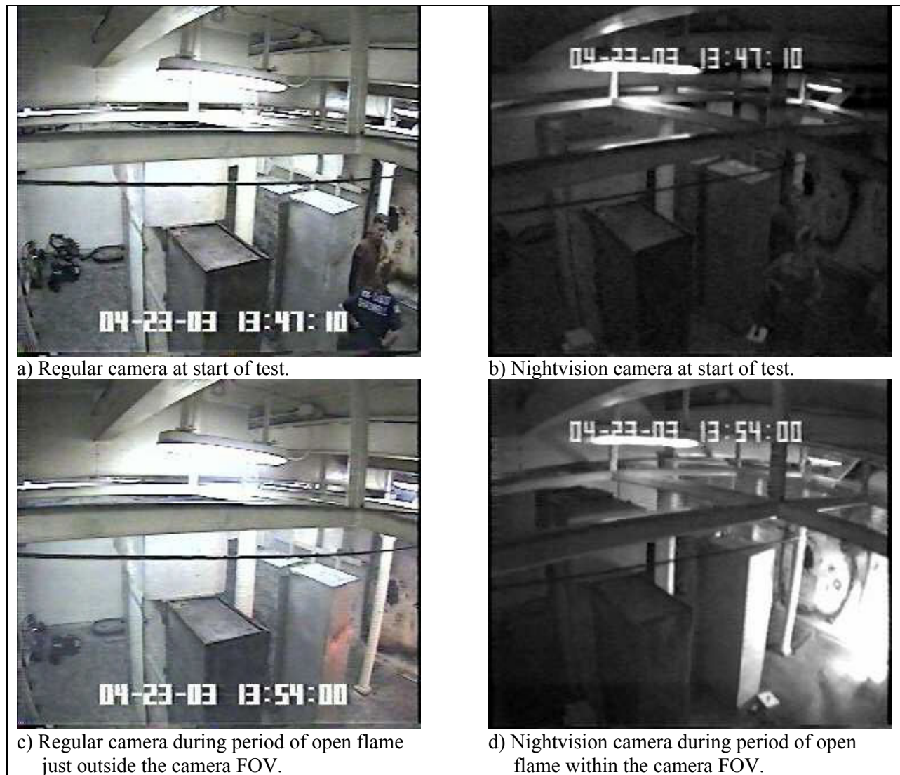
Fig. 5 – Camera video from VS1-21 test, camera position 3. Regular and nightvision still images showing the compartment before test ignition and during a flaming event within the nightvision camera FOV and nearly within the regular camera FOV
