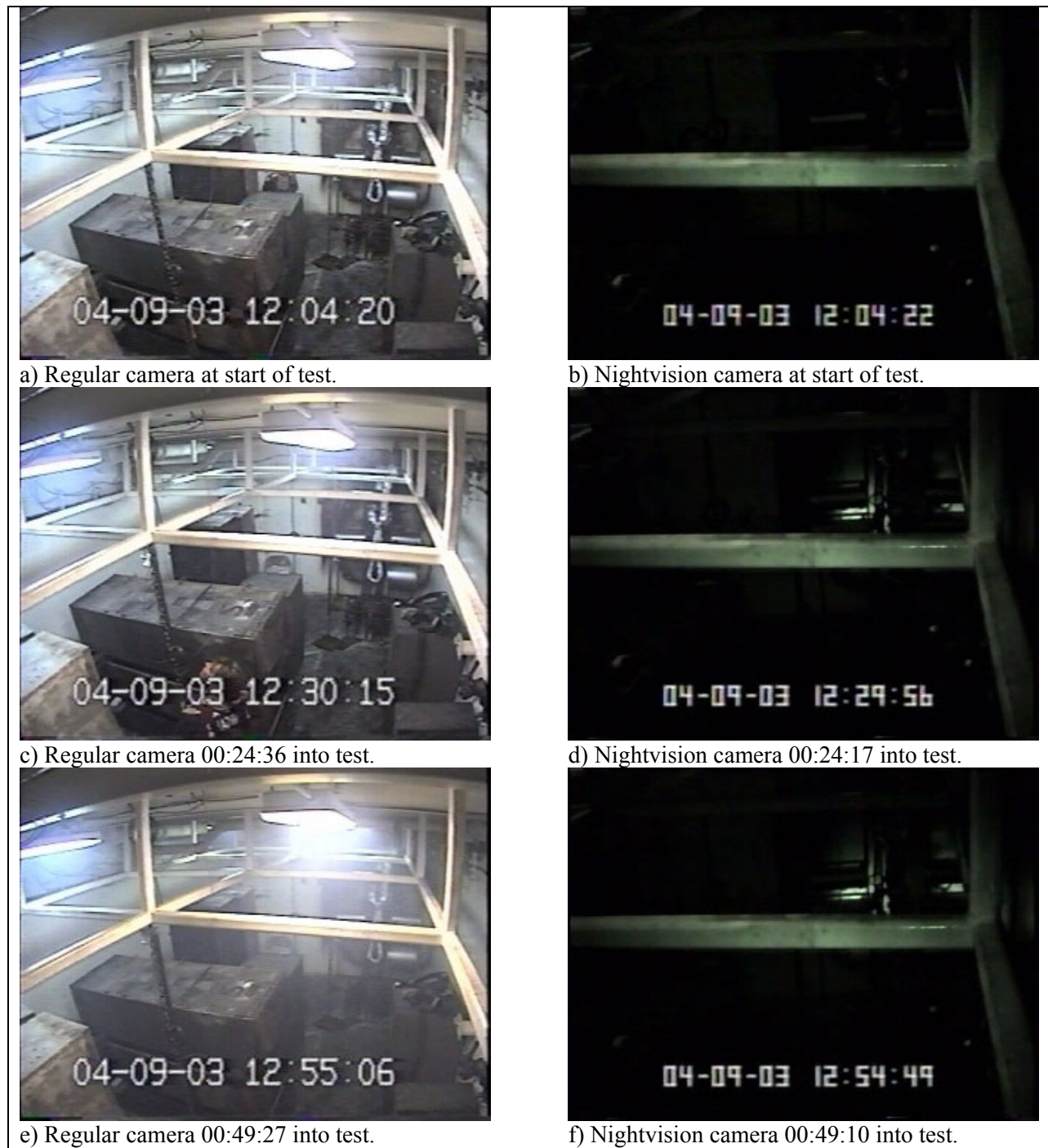
Fig. 8 – Camera video from CVNX-34 test, camera position 1. Regular and nightvision still images showing the compartment before test ignition and at two times during the test
