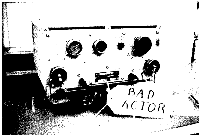
Base-level maintenance shops have tried a wide variety of tagging techniques to mark Bad Actor LRUs, but none are part of the "official" system.
