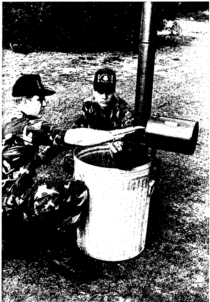
SrA Donald F. Inman Jr. (left), and Sgt Donnie L. Eubanks Jr., both of the Tyndall Prime RIBS team, prepare the immersion heater. (Photo by SSgt Rick L. Fligor)
