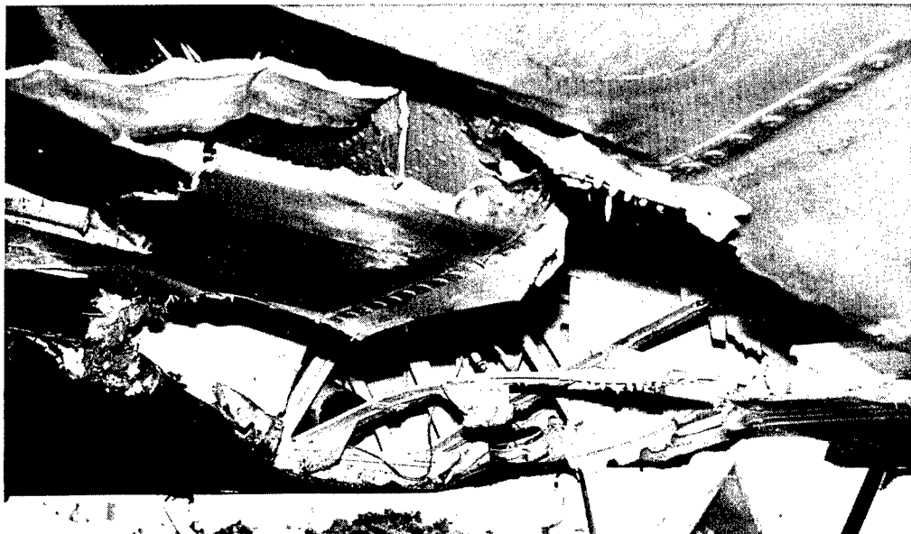
Damaged belly skin with severed longerons.
