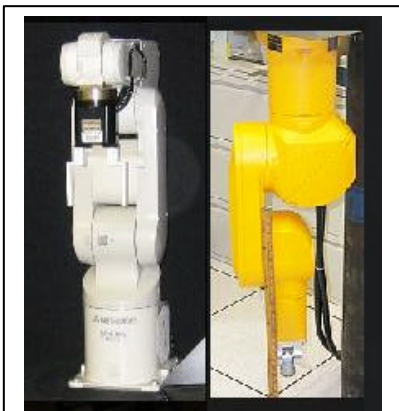
Figure 2.3: Mitsubishi RV1A robot arm (left) and Staubli RX60B robot arm (right)
