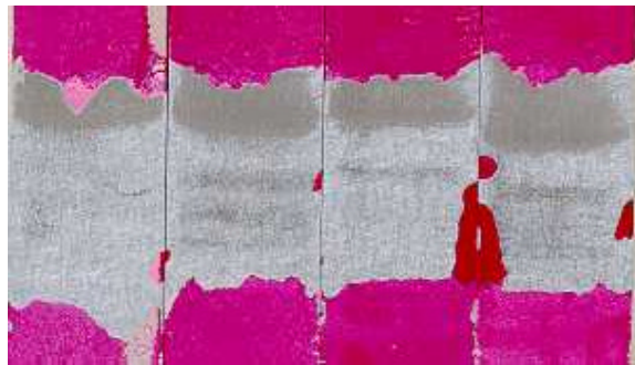
Figure 2.4-3: Failure Mode Exhibited Using Cloth-Applied Primer
