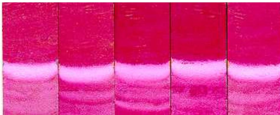
Figure 2.3-2: Failure Mode Exhibited by “Optimal” Nylon-Pad Deoxidized Specimens Treated with Boegel-EPII and Tested at 120°F and 95-100% Relative Humidity
