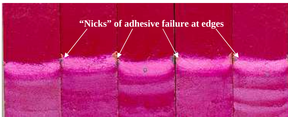
Figure 2.3-3: Failure Mode Exhibited by “Optimal” Nylon-Pad Deoxidized Specimens Treated with Boegel-EPII and Tested at 140°F and 95-100% Relative Humidity
