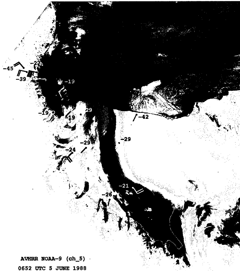
FIG. 16. Thermal IR image and AWS observations over the Ross Ice Shelf showing katabatic winds from glaciers in the Transantarctic Mountains and a katabatic surge from the Siple Coast (Polar Meteorology Group, BPRC).
