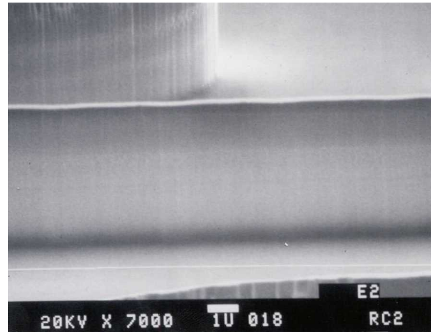
Reduced roughness using wet chemical etch after ICP etch
