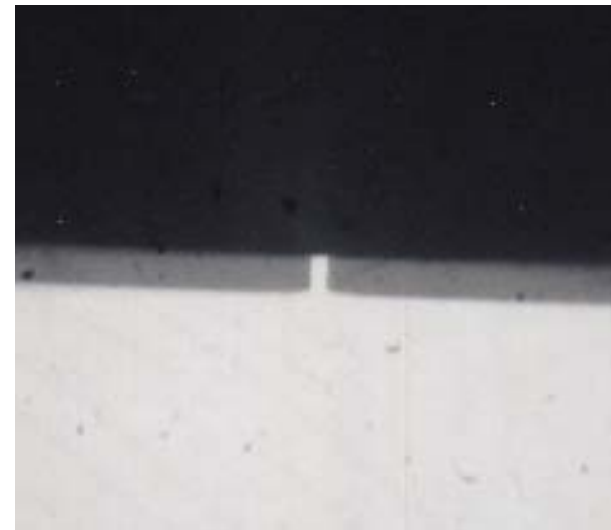
Cross-sectional view of BCB-planarized ridge waveguide
