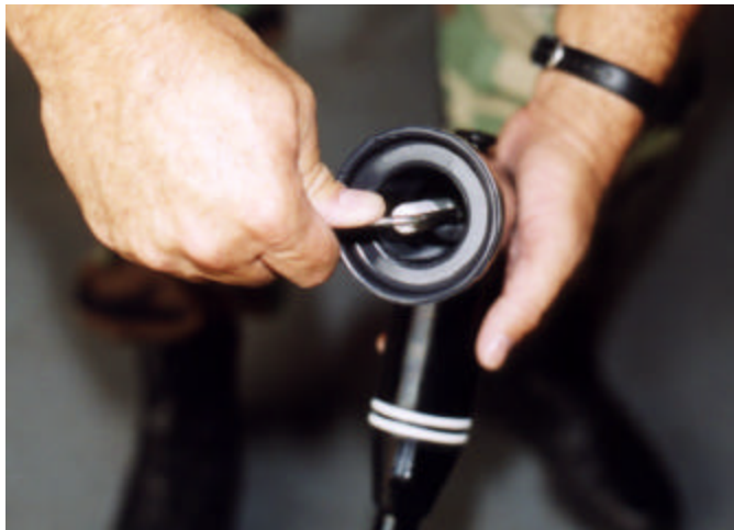
Figure A4.14. Short End of Wrench in Hole of the Probe.
