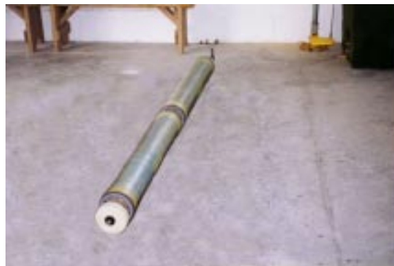
Figure 49. Puller Rod Inserted into R.O. Element String.
