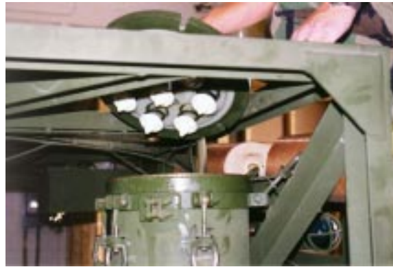
Figure 43. Cartridge Filter Cover Removal.
