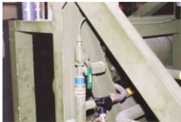
Figure 34. VENT PRODUCT WATER Valve.
