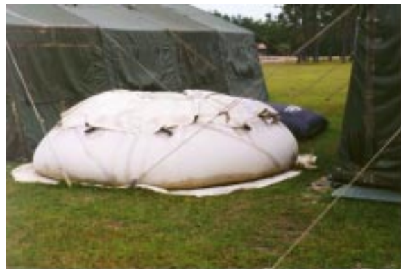
Figure 11. 3,000-Gallon Onion Tank.
