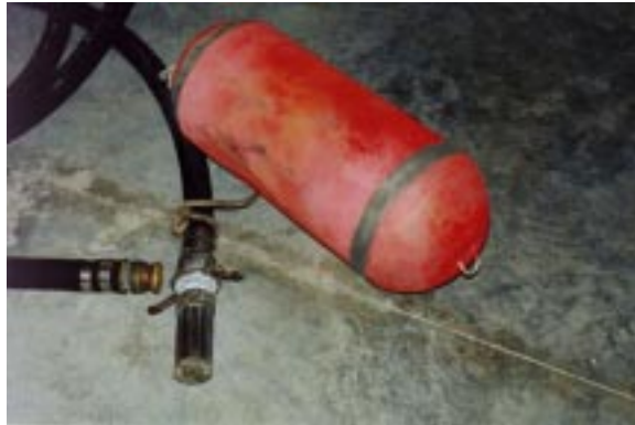
Figure 14. Strainer and Float.
