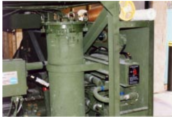
Figure 7. Reverse Osmosis Pump Assembly.
