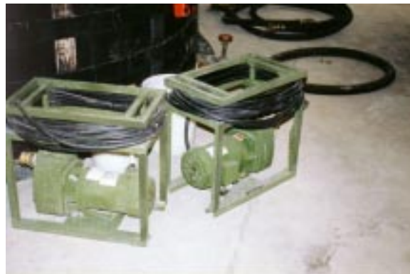
Figure 13. Raw Water Pump.
