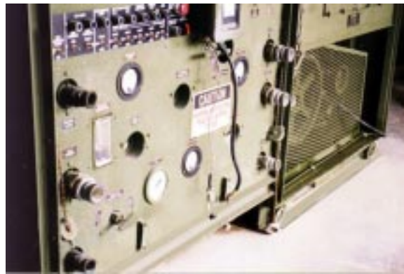
Figure 21. Quick Disconnect Fittings on Control Panel.
