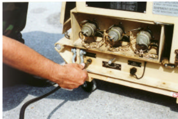
Figure 59. Quick-Disconnect Fuel Fitting.
