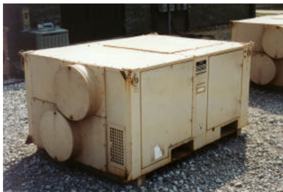
Figure 29. A/E32C-39 Environmental Control Unit.
