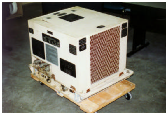
Figure 55. Mobile Water Chiller.
