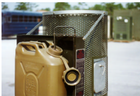
Figure 27. Siphon Assembly Placement.
