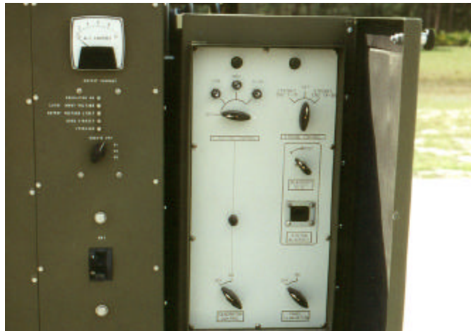
Figure 41. Backup Control Panel and Regulator Panel.
