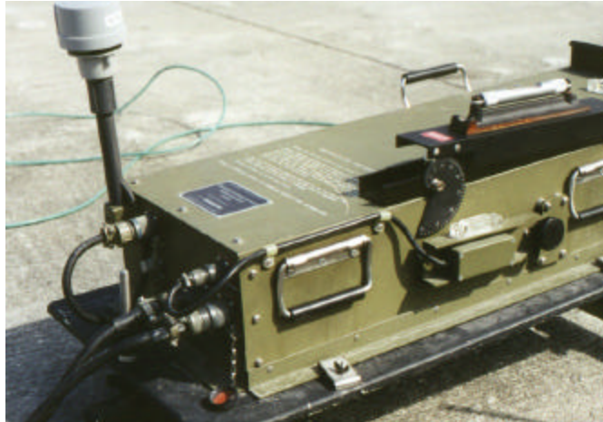
Figure 20. Inboard PAPI and Series Circuit Adapter.
