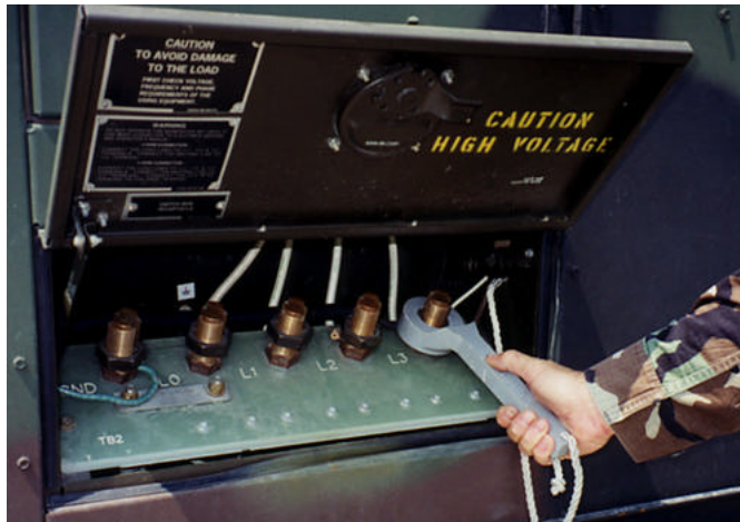
Figure 29. Generator Unit Power Cable Connection to Generator.
