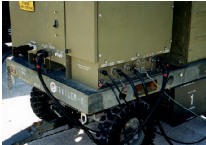
Figure 33. Cable Connections from Control Panel to Regulator.
