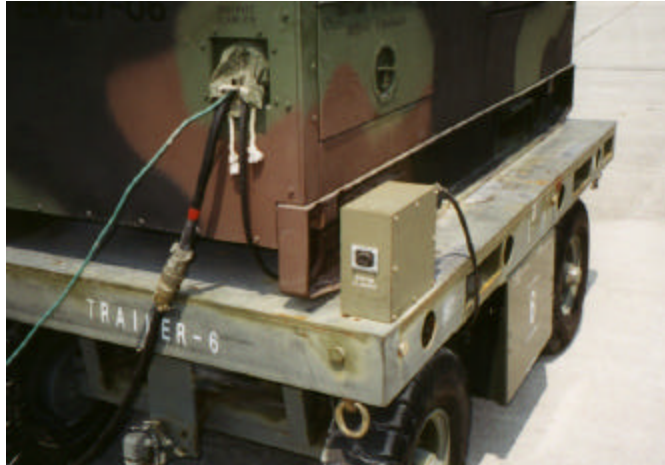
Figure 31. Generator Control Cable Connection to Generator.
