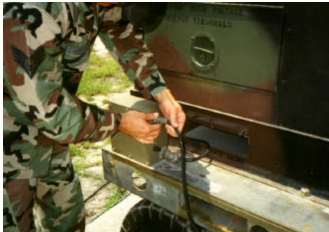
Figure 31. Generator Control Cable Connection to Generator.
