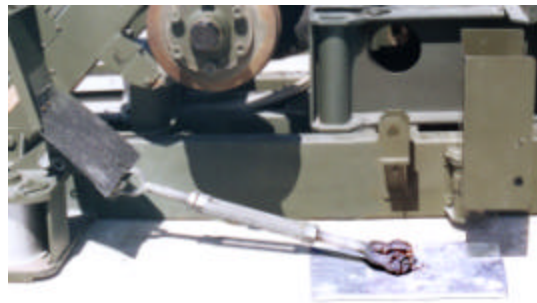
Figure 43. Right Rear Wheel Anchor Point Using a Triple Turnbuckle Fitting and Turnbuckle – Right MAAS Trailer.
