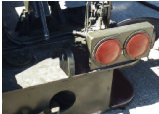
Figure 67. Right Front Anchor Point – Both MAAS Trailers (trailer shown raised only for clarity).
