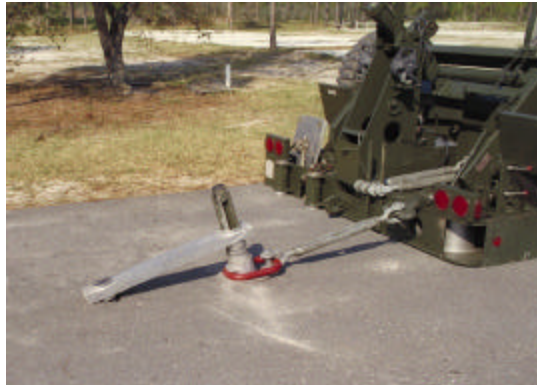
Figure 30. Install a Stake (Tie) Spacer on the Stake.
