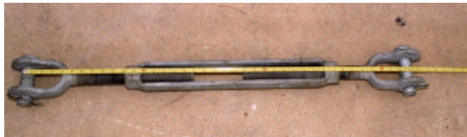
Figure 33. Adjust Turnbuckles to 39-Inch Length.
