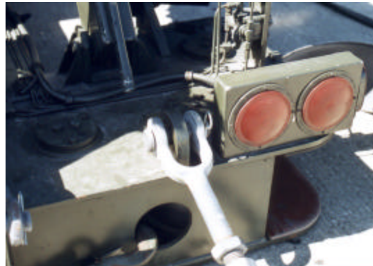
Figure 49. Right Rear Anchor Point with Turnbuckle – Both MAAS Trailers.
