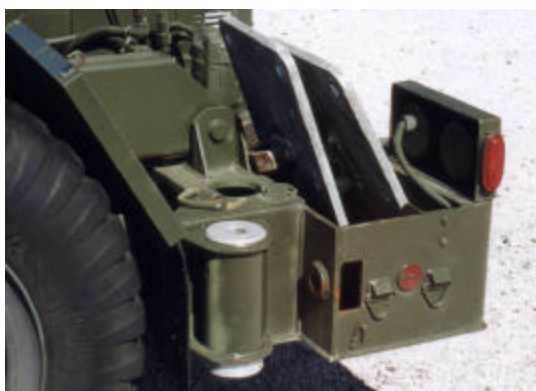
Figure 83. Right Rear Anchor Point – Both MAAS Trailers.
