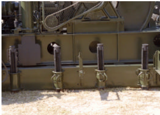
Figure 101. Proper Stake Orientation with the Body.
