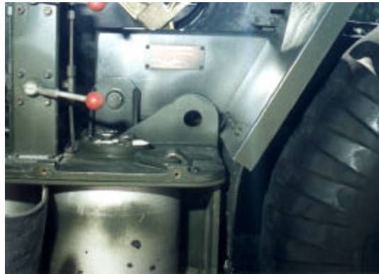
Figure 46. Anchor Plate Connection at Right Rear Wheel.
