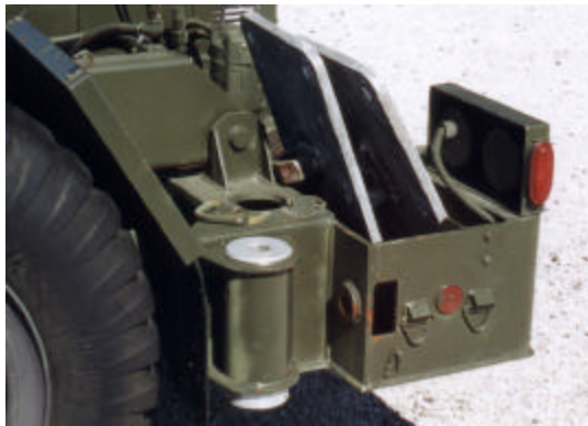
Figure 93. Right Rear Anchor Point – Both MAAS Trailers.
