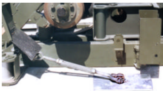
Figure 52. Typical Anchor Plate Location For Bi-directional Installation.
