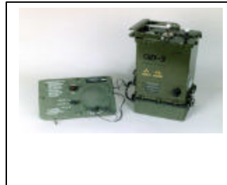
Figure 10. Example Detection Capability (CAM and M22 ACAA).
