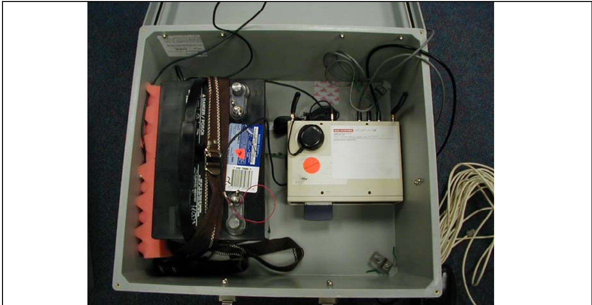
Figure 13-3 BAE Systems Test Bed Node Configuration
