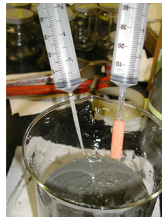
Figure 1. Syringes with filtration devices for porewater extraction by vacuum: left – stainless steel filtering medium; right – ground silica air stone filtering medium.
