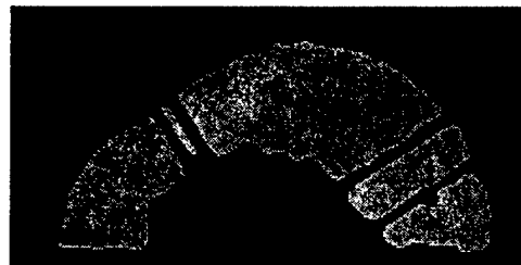
Fig. 10. Measured visibility modulus of Vega. Vega has an angular diameter far smaller than the diffraction-limited resolution of the Hale 200" Telescope, so the visibility modulus should be uniform across the upper quadrant. The measured visibility modulus agrees well with this expectation.
