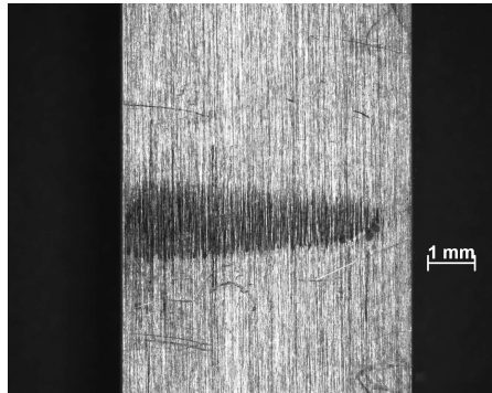
Figure B.1. Specimen #1 with P_{\text{const}} = 315 kN/m and Uni-Directional Shear
