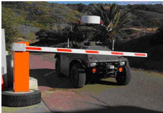
Fig. 4. MDARS Approaching Legacy PSE Swing-Arm Gate
