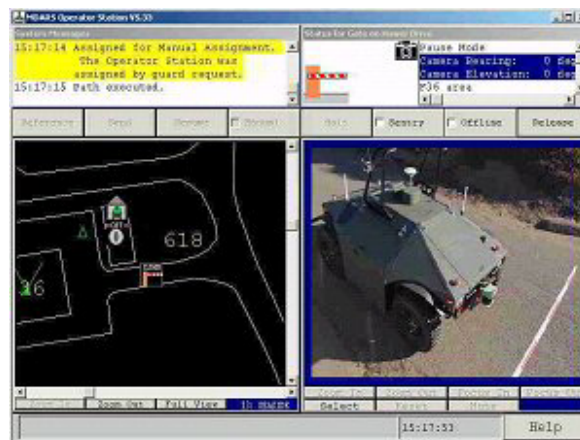
Fig. 6. MRHA Operator Station Controlling MDARS and Legacy PSE Swing-Arm Gate
