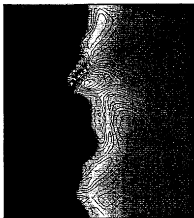
Figure 2 LES of premixed flame interaction with incoming turbulence. (a) Vorticity and temperature contours, (b) vorticity and soot mass fraction contours. Soot production within a 2-3 LES-resolved flame is captured within the subgrid LEM in these LEMLES studies.
