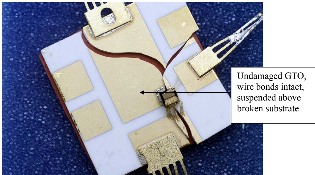
Figure 1. Results of poor thermal conductivity. (SiC GTO thyristor on alumina module.)
