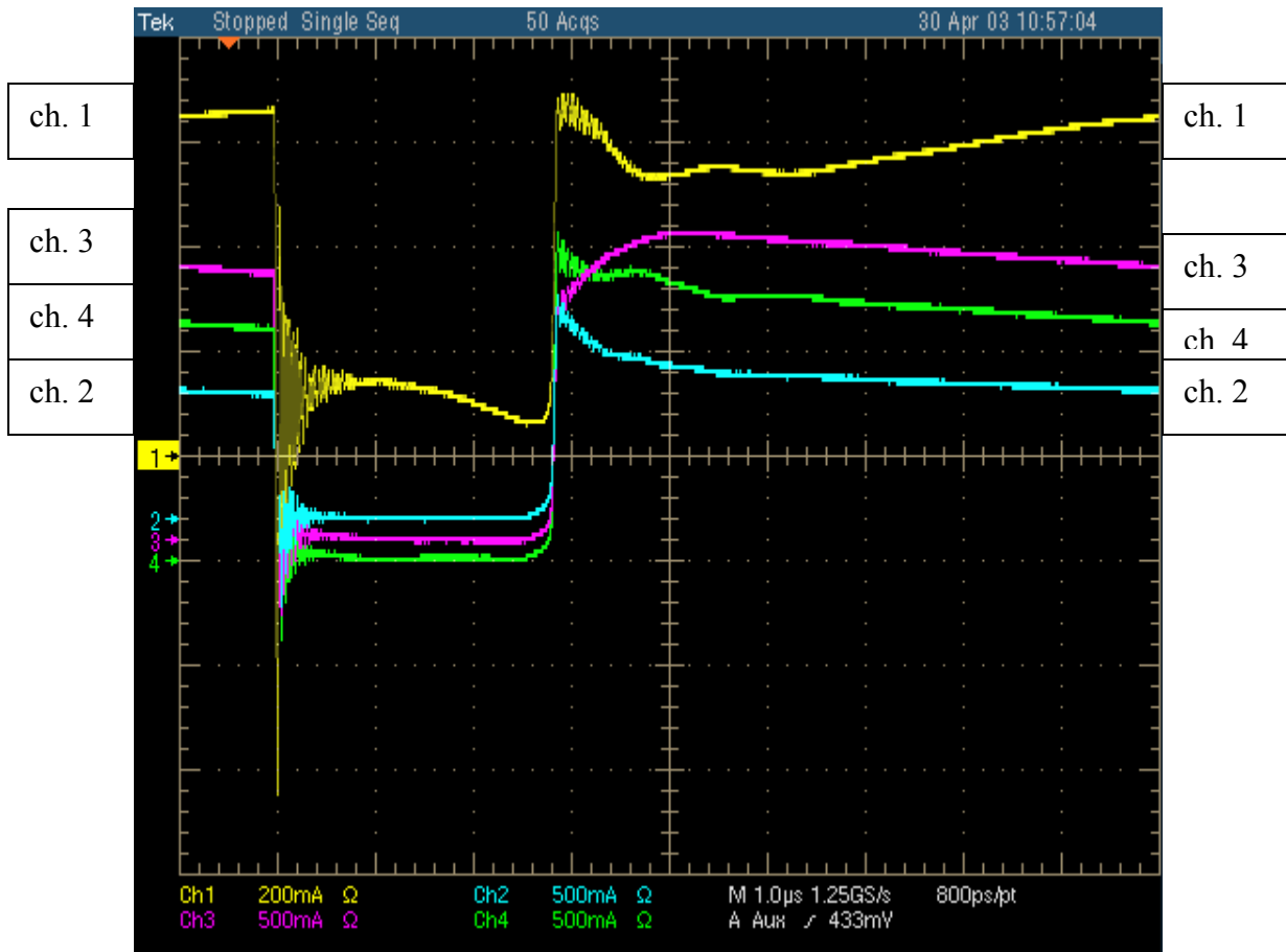
Figure 9. Diodes JBS1, JBS2, JBS3, and JBS4 in parallel.
