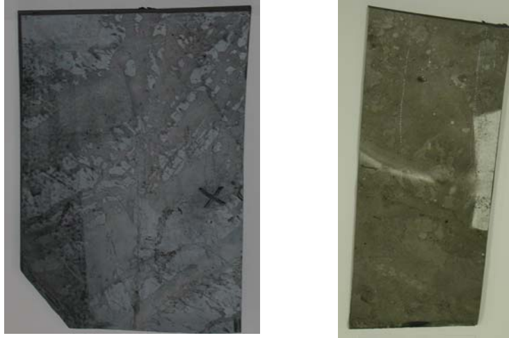
Figure 1 Photographs of two samples (1W-T-6, 1W-T-1) from top-side of Wing Box 1 (1 minute exposure)
