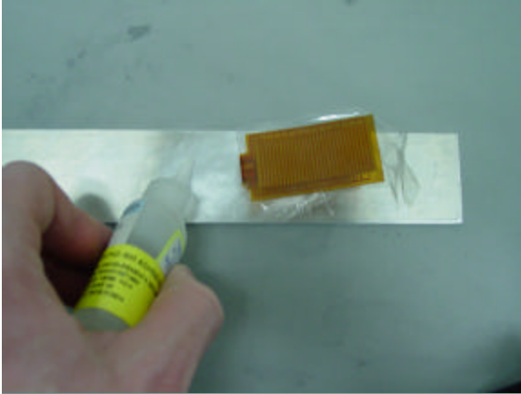
Figure 21-i. Application of Bonding Agent. M-Bond 200 squeezed onto specimen surface in thin, parallel lines to ensure complete coverage of the underside of PZT.
