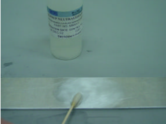
Figure 21-f. Neutralize. M-Prep Neutralizer 5A thoroughly applied to area with cotton swab. Area wiped once with clean cloth.
