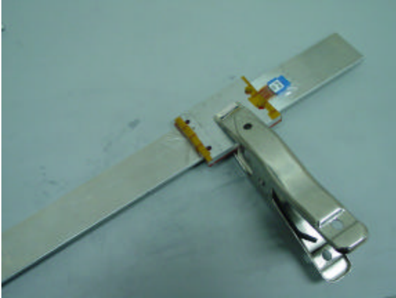
Figure 21-j. PZT Placement and Clamping. PZT immediately folded over and visually checked for complete coverage of M-Bond 200 on bottom surface. Excess bonding agent is squeezed out from under PZT and wiped away. Clamp used to ensure constant pressure throughout drying time. Aluminum block diffuses pressure over entire PZT and alleviates direct contact between clamp teeth and actuator. Allowed to set for 15 minutes.
