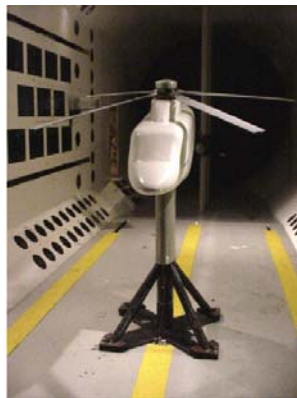
Figure 24: ATR system mounted on the ARES helicopter testbed with in the TDT.
