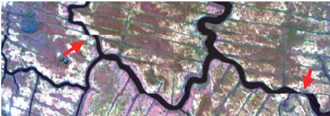
Fig. 11 — Portion of an image showing two discontinuities (the locations are highlighted by the red colored arrows) apparently caused by “dropped lines” (lost data). The dropped lines appear to occur mainly in the high frame-rate (46 fps) 1-m spatial resolution data.
