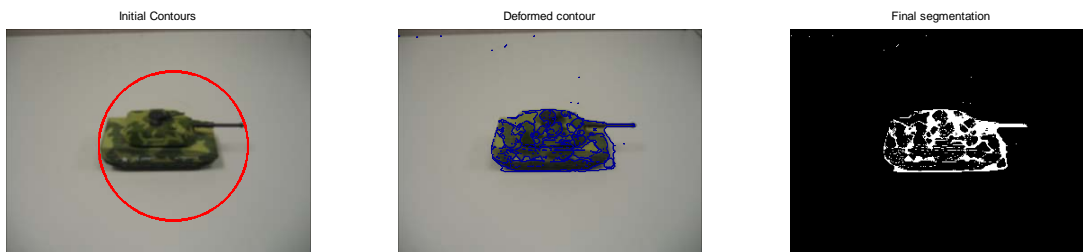
Figure 12 Color snakes applied into the RGB image in Figure 6 (258x253x3). (Left) A contour is initiated at the exterior of the object. (Middle) (Right) Color snakes find many internal boundaries because of camouflage paint.
