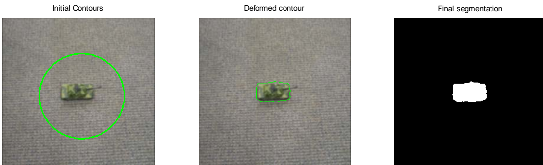
Figure 24 Rousson-Deriche model applied into Figure 7 (258x253x3). (Left) An initial contour is placed manually at the exterior of the object. (Middle) The contour moves towards the object and stops on the boundary of the object. (Right) The image is divided into two sets; the object and the background.
