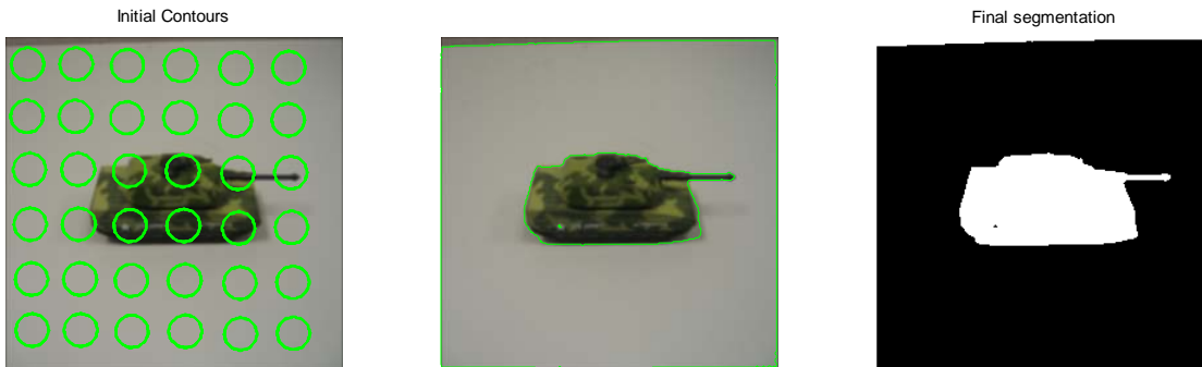
Figure 17 Chan-Vese model applied into the RGB image in Figure 6 (258x253x3). (Left) 36 initial contours are placed using distributed seeds. (Middle) Active contours move towards the boundary of the object and the boundary of the image. (Right) The image is divided into two segments; the object and the background.
