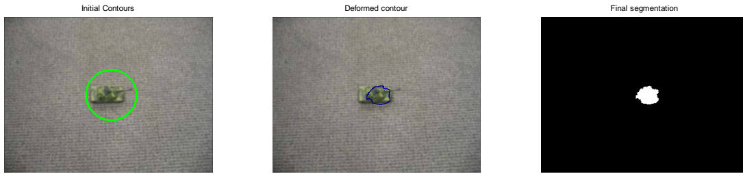
Figure 9 Geometric active contours applied into Figure 7. (Left) The initial contour is placed at the exterior of the object. (Middle) (Right) The contour keeps shrinking even after crossing the boundary of the object.
