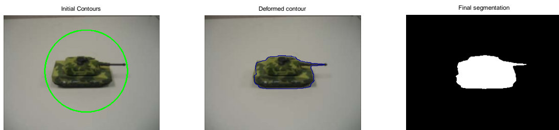
Figure 8 Geometric active contours applied into Figure 6. (Left) An initial contour is placed at the exterior of the object. (Middle) The contour stops at the boundary of the object. (Right) The image is divided into two segments; the object and the background.
